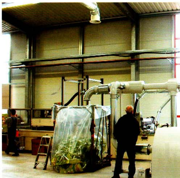
In the original installation the edge trims were collected in big bags
