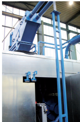
Picture 7: View of the sound hood and the material separator
