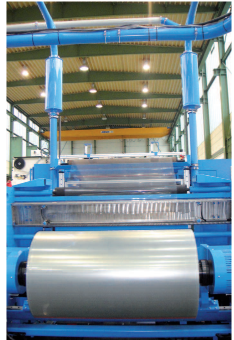
Picture 1: View of the Suction line from the parent roll
