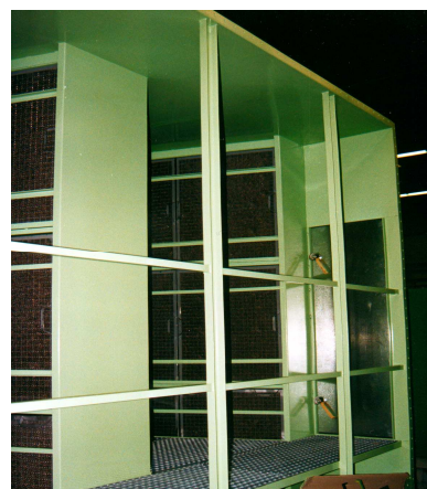
Fig. 2: Inside of the Oil / Emulsion Mist Separator KG
