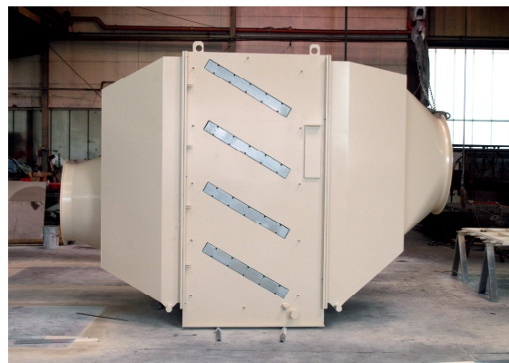
Abb. 2: Oil / Emulsion Mist Separator in the final inspection
