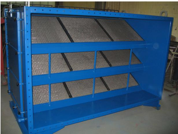
Fig. 1: Inlet of the Oil / Emulsion Mist Separator KK
