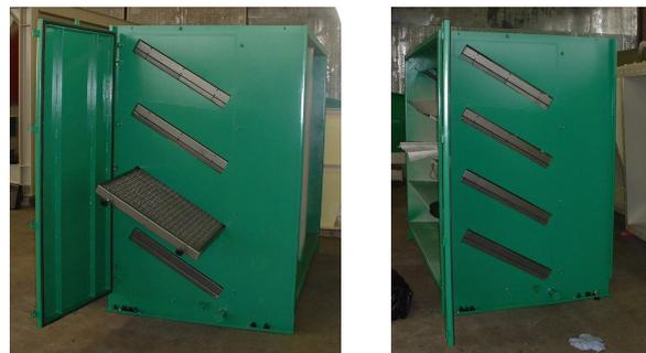
Fig. 2: Oil / Emulsion Mist Separator KK in the final inspection
